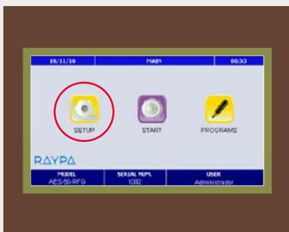
1. On the autoclave screen, enter the "SETUP" menu.
