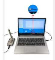
4. Upon completion of cycle, recover the data logger from the sample and insert on the connection base again while the latter is connected to a PC. Using the software, view on screen and/ or export data obtained during cycle.
