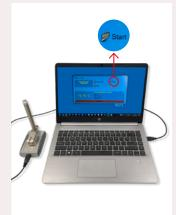
1. Connect the data logger to the connection base, and connect the latter to a PC. Download and install the free software to start recording data by clicking on "Start".
